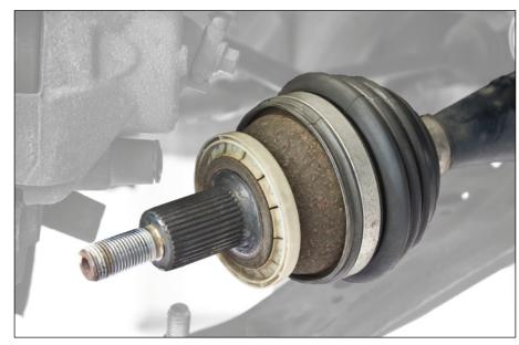
Figure 1: The Sealing Rings could differ in design and color!
